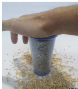
Figure 4. Press the feed down
