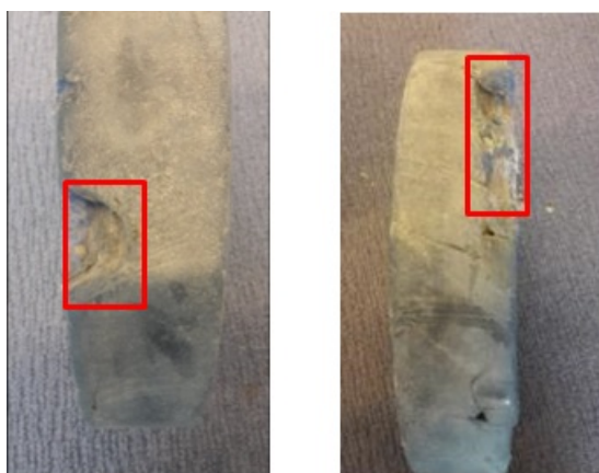
Figure 102. Too much wear on swivel wheel
